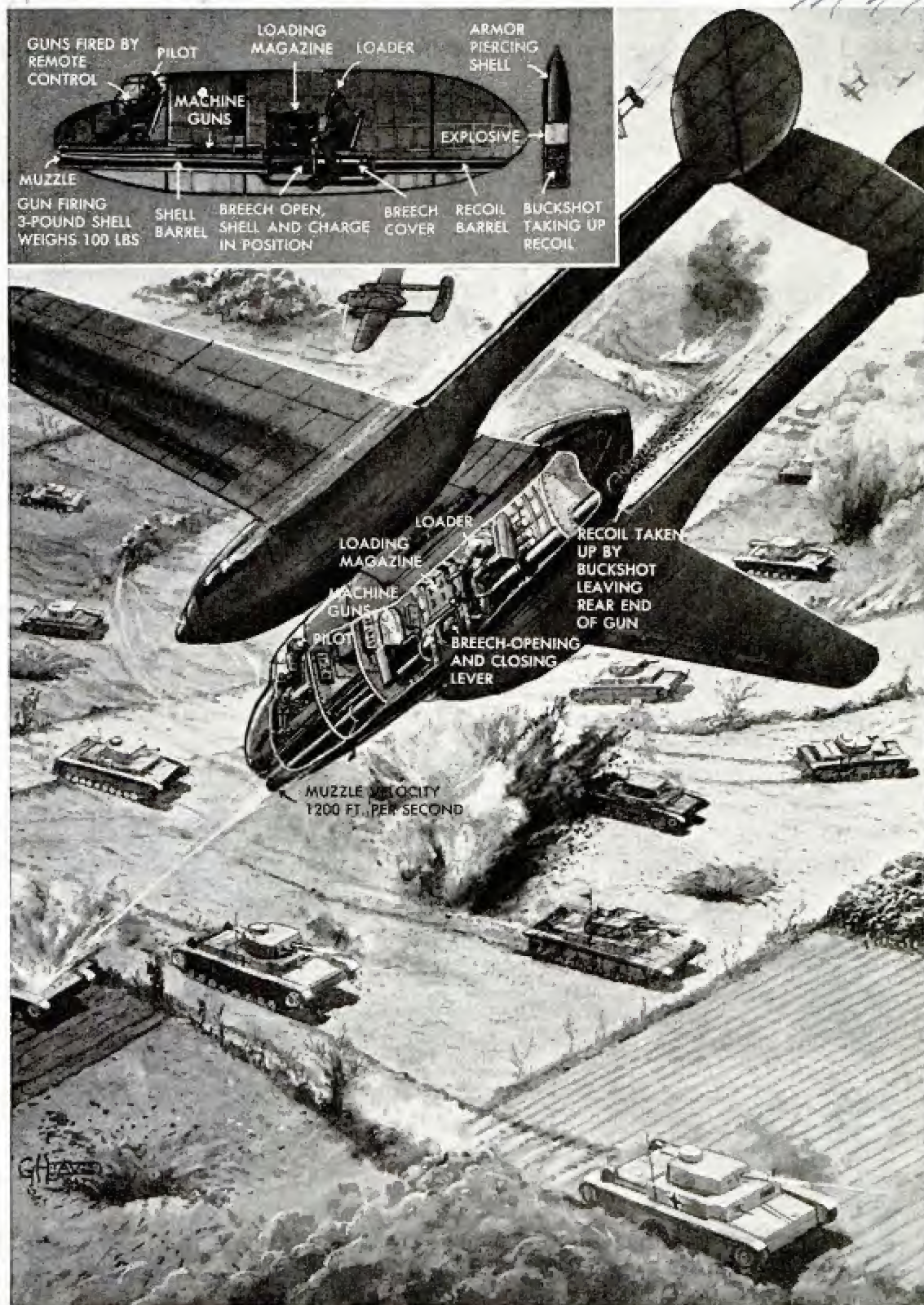
Warplanes of the future may fire three-inch and larger shells, if development of the Davis nonrecoil gun, proposed in England, proves successful. Its barrel extends to front and rear of the plane, and the shell, with its charge at the center, provides for a "backfire" of buckshot to absorb the shock. Such guns, tried years ago, developed a muzzle velocity of 1,200 feet per second
